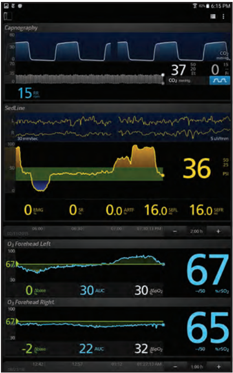
Kite displays data from modules connected through MOC-9 ports to Root, such as SedLine, O3, and NomoLine
