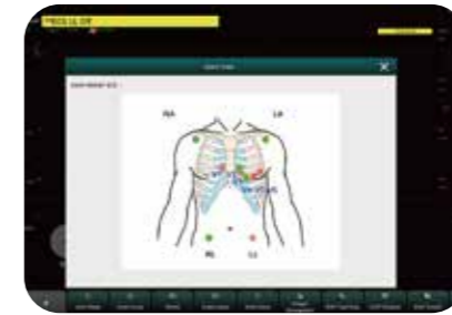
ECG lead alarm warning shows the off lead position clearly
