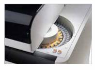
Covered sampling system All cover closed during testing , sample disk can be partially opened when needed
