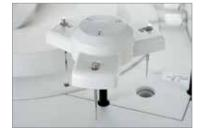
Effective mixer unit Individual mixer units for reagents and samples. Threehead mixing bars perform more effective mixing. Two grade washing reduces contaminant significantly
