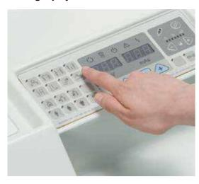
Simply select one of the 72 preset anatomical programs (APR) to configure the optimal radiography conditions for the corresponding radiography region, direction, and body thickness.
